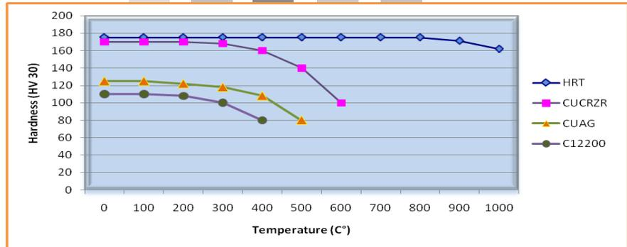
While the introduction of different tip materials may improve wear resistance in certain applications, the harder material with a higher annealing temperature sacrifices electrical conductivity which can lead to poor arc starting characteristics.
