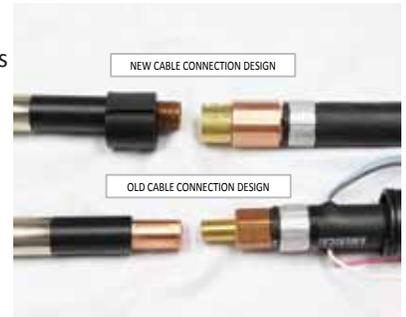
We are making the conversion process as painless as possible or our customers. All replacement semi-automatic goosenecks will incorporate a dual male and female thread to accomadate the old and new cable system. All replacement cables will be shipped with an adaptor to convert to older style goosenecks.
